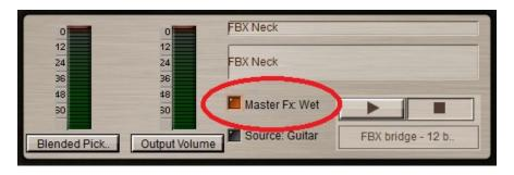
When set to Dry, this button is a global bypass for *all* effects. The Firebird X output comes solely from whatever pickups you have selected and there is no processing. Although you cannot edit any effects when set to Dry, you can select different magnetic pickup configurations.
