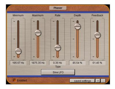
**Minimum:** Sets the phaser sweep's lowest frequency limit. **Maximum:** Sets the phaser sweep's highest frequency limit.
