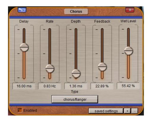
**Delay:** Sets the fundamental range covered by the effect. Shorter delays are for flanging, vibrato, and resonators, while longer delays work for chorusing and ADT.
