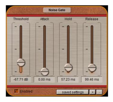
Threshold: Signals below this level are blocked (i.e., the gate is "closed").
