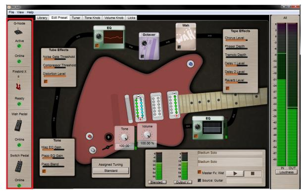
**G-Node Active:** Blinks green to indicate the G-Node is communicating with Firebird X. **G-Node Online:** The G-Node is connected to your computer and communicating via USB 2.0. **Firebird X:** This indicator alternates between Offline and Connecting if Firebird X is unplugged. Once connection is complete, the indicator lights green, stays lit, and says Ready.
