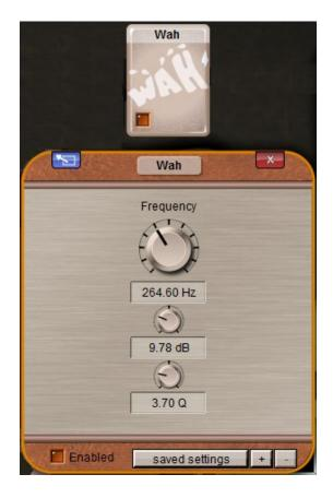
**Frequency:** Sets the bandpass filter's center frequency. The pedal controls this parameter. **Filter Gain:** This parameter, directly below the Frequency control, determines the boost amount at the selected frequency.
