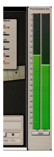
The left meter always shows the level at the Tone Block output (e.g., the mixed sound of all selected pickups), while the right meter always shows the final FBX output.
